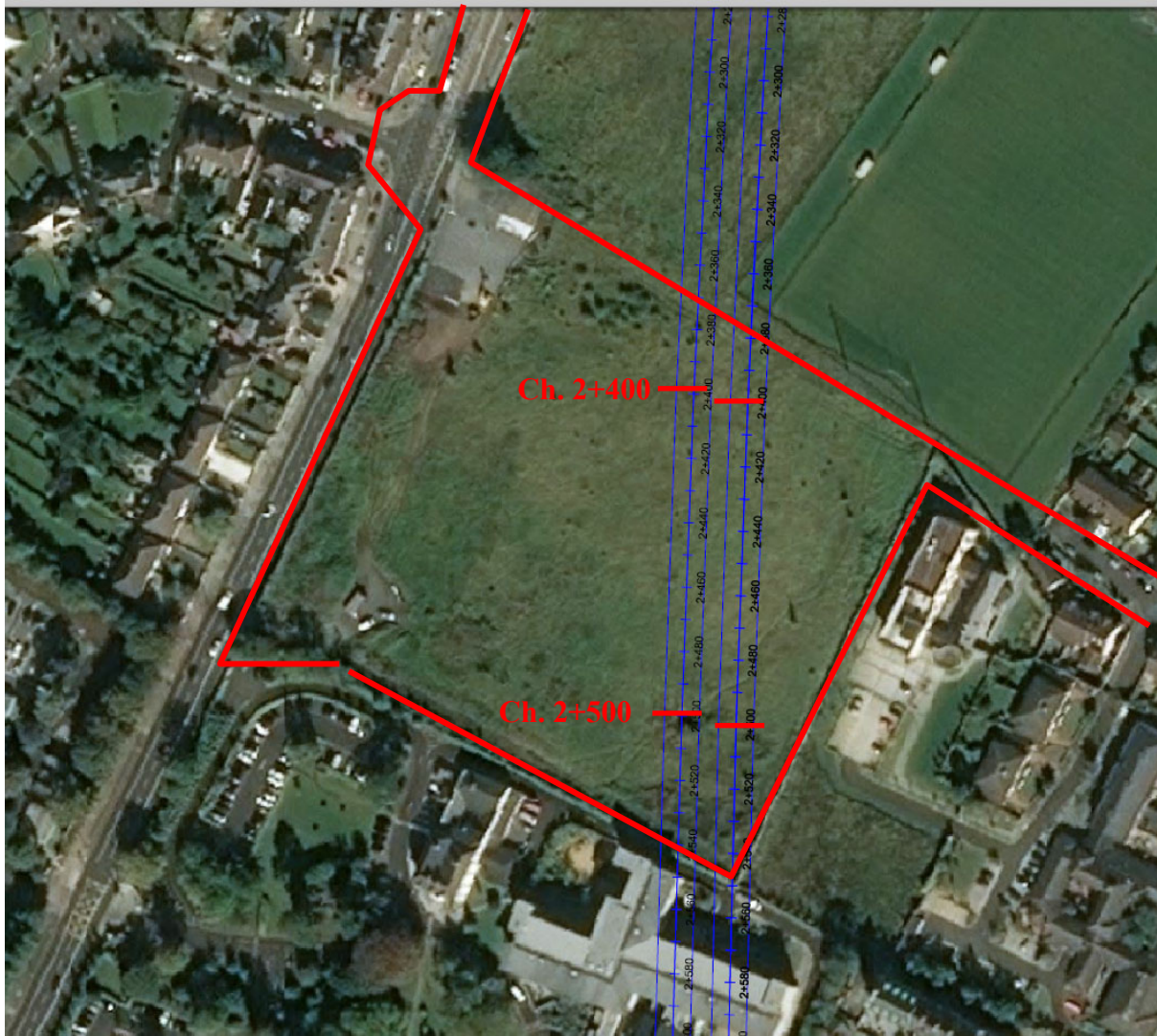
Figure 4-1: Plan View of DPT in the vicinity of the site showing tunnel chainages (site shown in red)
